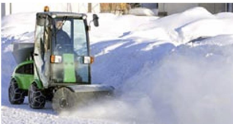
*Adaptable vehicles are available which will fit cycle paths. Just over 1m wide, this machine can clear snow, spread salt, wash, sweep paths and collect leaves*
