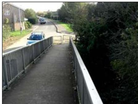
Right-angle bend (top) and chicane at Milton end (to be removed) of the substandard footbridge linking Milton to the new Park & Ride site.
