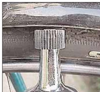
*Make sure dynamo lights are mounted correctly. 'Bottle' dynamo rollers should run against the 'track' on the tyre.*
