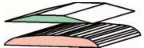
The shape of a national standard central delineator strip (top) and of the sub-standard raised white stripe as measured beside Shelford Road (bottom). The steep edges can be dangerous in wet weather.
