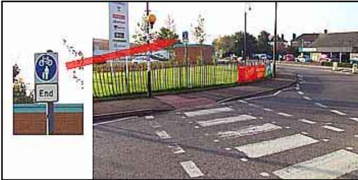
*Councillors were placated after being told cyclists could legally use this inadequate pavement. In fact, the signing shows that shared-use ends 3 m short of the roundabout that needs to be avoided.*
