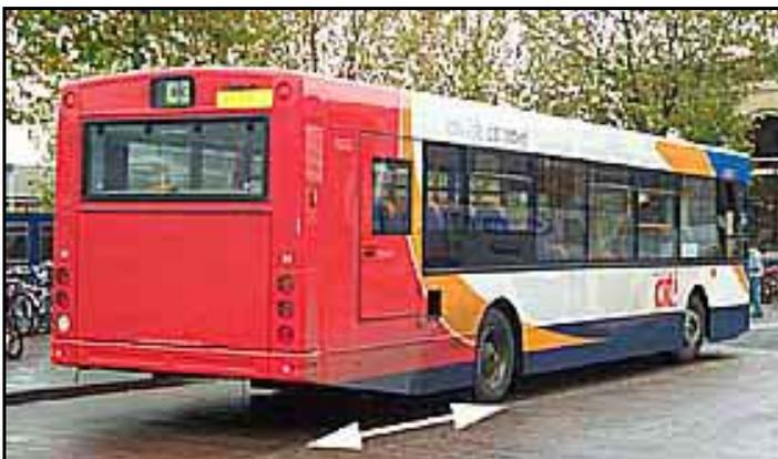
large rear overhang of some 3.5 metres and the lack of experience of many bus drivers. When such a vehicle makes a sharp turn in a confined space the driver may apply full lock from stationary and then move off. This causes the rear of the vehicle to move sideways in the *opposite* direction to the front. This rear kick out can be as much as 0.8 metres. The bus driver is not always aware of this danger – I've witnessed a bus damaging the side of a stationary car like this, and the bus
