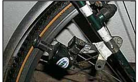
*The Nordlicht 2000 generator. This specimen doesn't work in the rain, and it doesn't even work on damp roads in freezing weather. Poor value at £20, and without it, £43 of lights aren't working either.*
