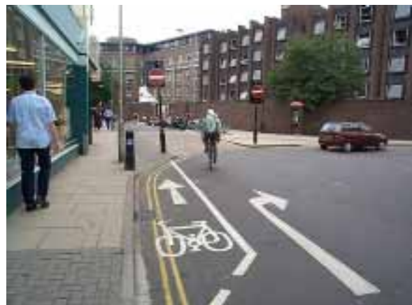
Left: St Phillip's Road. Parking close to the far cycle gap has rendered it unusable. This is cycle exemption at its most complicated and expensive.
