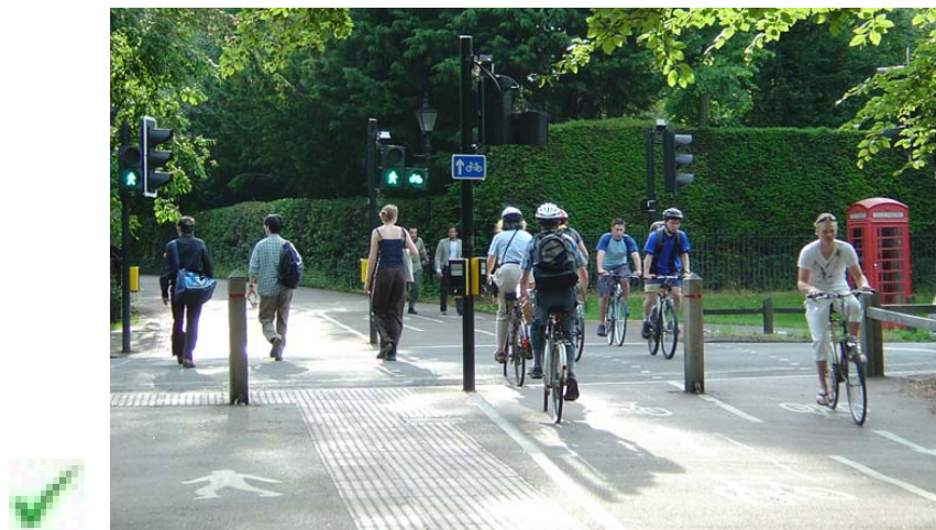
Queen's Road: Pedestrians and cyclists are informally separated. Barriers are few. Bikes are detected automatically. Signals are visible opposite. Everyone can cross easily without running into each other.
